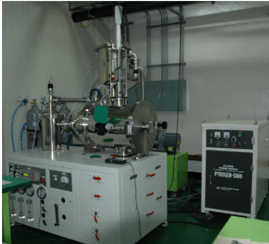
Fig. 1. DC plasma reactor system for the synthesis of SiC nanopowders.
